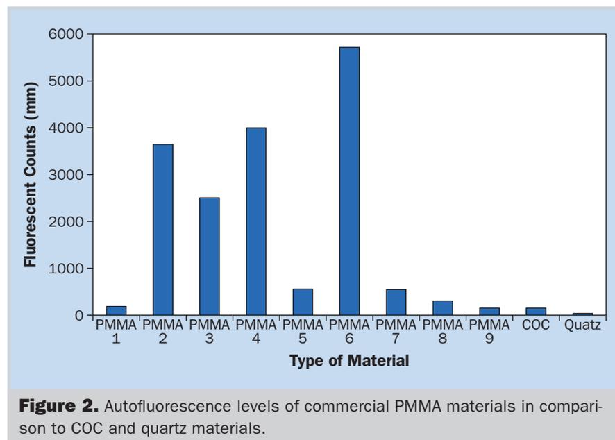
**Figure 2.** Autofluorescence levels of commercial PMMA materials in comparison to COC and quartz materials.
