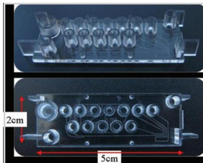
**Figure 1.** Disposable PMMA microfluidic chip (45-degree-angle side view and top view) made by injection molding. Various wells are used for placing electrolytes, the sample, and conjugated antibodies.
