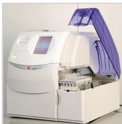
**Figure 9.** An automated instrument that samples, mixes, reacts, concentrates, and separates analytes using PMMA disposable chips by the EATA method.
