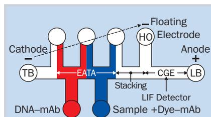
**Figure 4.** A schematic diagram showing the well and channel layout on the PMMA microchip. LB is the buffer containing the leading ions; TB is the buffer containing the trailing ions. The HO (handoff) well also contains LB. DNA-mAb is anion-bound human anti-AFP antibody; dye-mAb is fluorescent dye-bound human anti-AFP antibody (mouse monoclonal antibodies).
